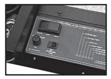
With the mode switch in AUTO, press the EXERCISER switch. Hold it down for at least 10 seconds and release. The generator should start within a few seconds. The unit will run for about 12 minutes before shutting itself down automatically.
